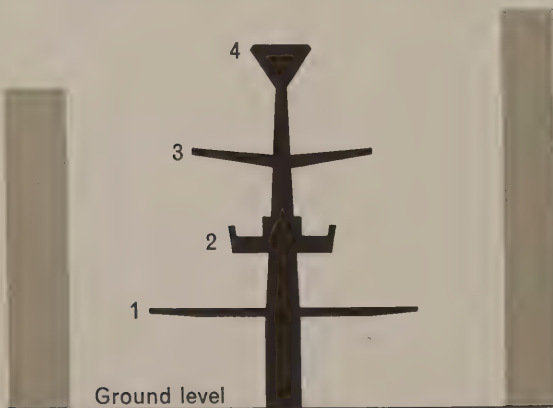
206 The proposal by Mr Rigby Childs for a free-standing pedestrian walk in Oxford Street. This is a cross-sectional view with existing buildings on either side. The ground level would be wholly available for two carriageways of traffic. Level 1 is the pedestrian platform. Level 2 is the two-way travelator with canopy over at 3. At level 4 there is a longitudinal structural member for stability.
